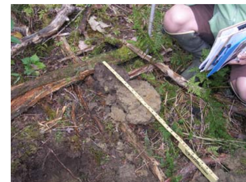
Left- measuring color contrast in soil sample
