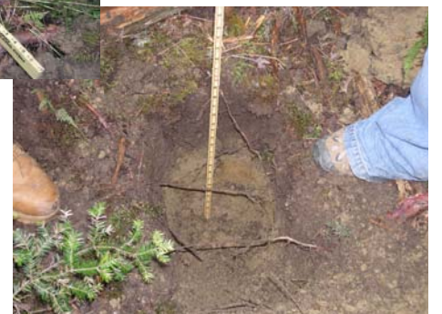
Below - Measuring soil contrast and pit dept of test hole, checking for wetness
