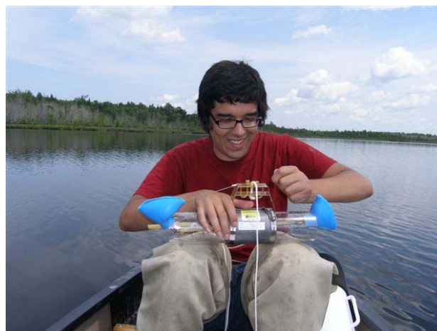
Photo of Isaac St. John preparing a Van Dorn sampler, which collects water from a pond or lake at deep depths.
