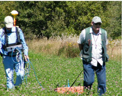
(left) J. Doolittle NRCS and Matthew Edberg using GPR to study proposed cemetery site (below) GPR screen
