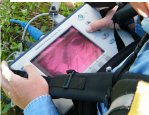
(left) J. Doolittle NRCS and Matthew Edberg using GPR to study proposed cemetery site (below) GPR screen
