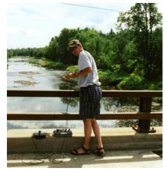
Dave Joseph measuring dissolved oxygen (DO) from the Livery Br.
