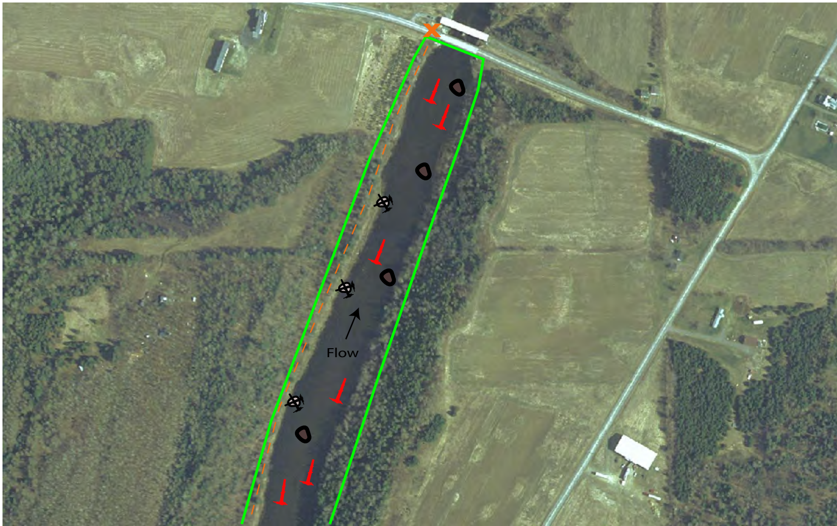
Sheet 3. Conceptual restoration design planview for the Covered Bridge Geomorphic Assessment Site (1 of 7).
